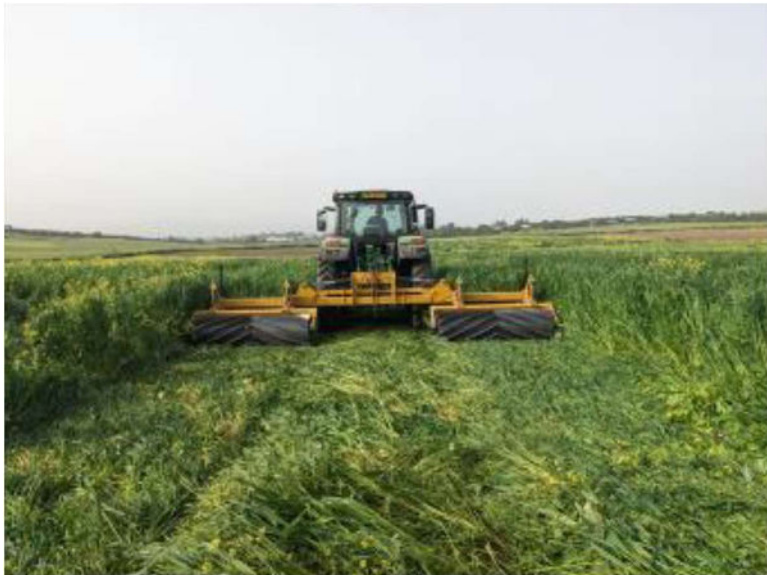
Crushing of the biomass with the help of the roller-crimper
