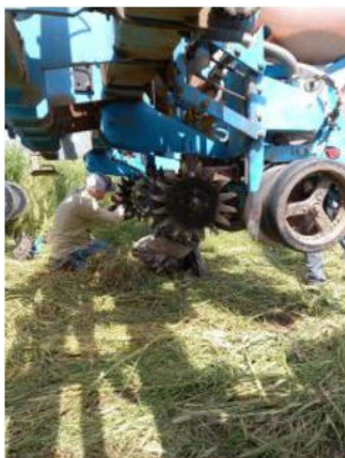
Finger weeders for removing vegetation from the sowing strip
